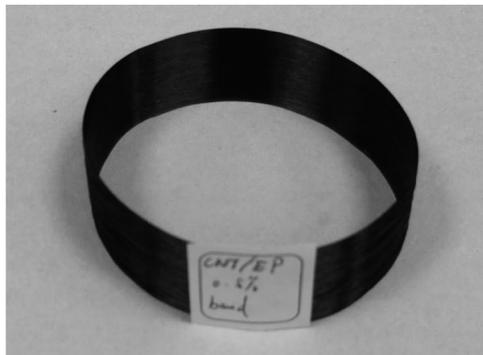
**Figure 10.** Unidirectional SWNT-reinforced epoxy laminate made using a translating mandrel and reactive spinning.
